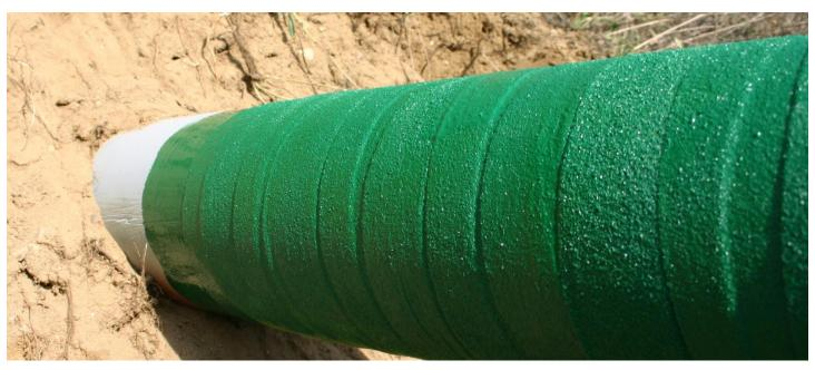
**Description:** A two part liquid epoxy saturated into a synthetic carrier designed for long term corrosion protection to metal structures. This epoxy composite wrap is designed to be used in place of wax wraps or traditional epoxy coatings. E-Wrap can be used for aboveground or belowground applications and is designed to protect pipelines in high stress environments caused by pipe movement, soil stress, thermal cycling, and transition areas. (available in multiple colors.)
